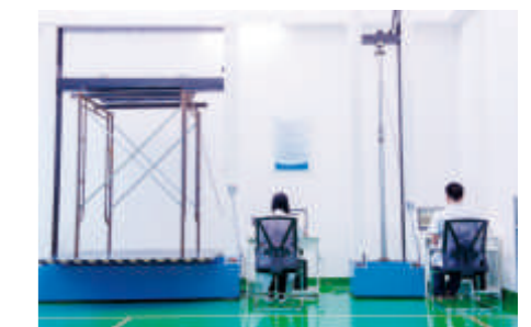
WDW-100微机控制电子抗压试验机 WDW-100 computer-controlled electronic compression testing machine
